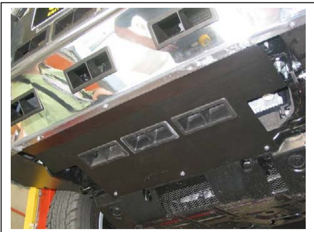
Figure 17: Centre under body guard fitted.
